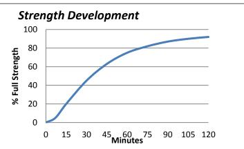
Graph shows typical strength development of bonded components at 23°C. Curing at higher or lower temperatures may affect cure speed.
